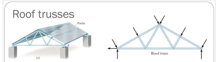
Load on roof transmitted to purlins, and from purlins to roof trusses at joints.
