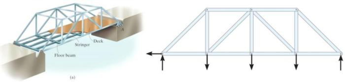
Load on deck transmitted to stringers, and from stringers to floor beams, and from floor beams to bridge trusses at joints.
